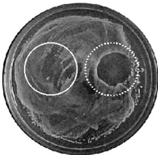
Figure 14 PP film (surrounded by a continuous line) and PP-g-AA with 12.9% grafting and natamycin (surrounded by a discontinuous line). There was a clear zone of yeast inhibition under the film containing natamycin.
