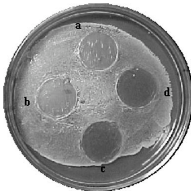
Figure 13 (a) PVC film and (b) PVC-g-AA showing no inhibition of the growth of yeast and (c,d) PVC-g-AA with 19.5 and 34.1% grafting, respectively, containing crystal violet and showing zones of inhibition of yeasts under discs. In all cases, the discs were removed to see the yeast beneath them.
